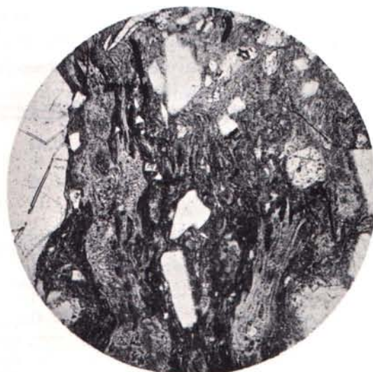
FIGURE 22. Collapsed pumice fragments in welded crystal-vitric tuff of the Windous Butte Formation (lower member). Plane light.
