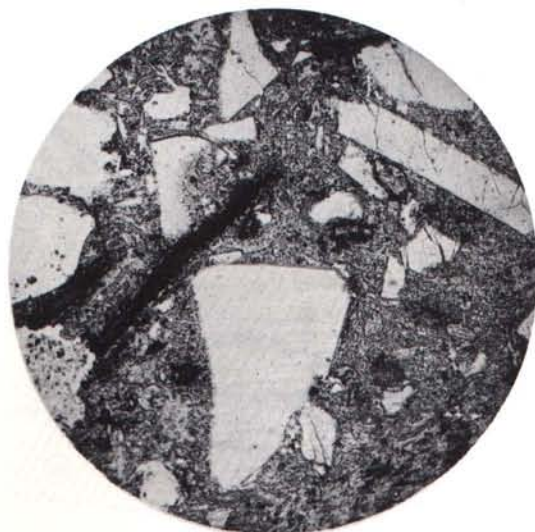
FIGURE 13. Partly devitrified (crystallized) groundmass in crystal welded tuff of the Windous Butte Formation (upper ignimbrite). Plane light.
