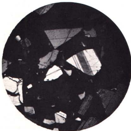
FIGURE 21. Angular crystal fragments in welded crystal tuff of the Windous Butte Formation (upper member). Crossed nicols.
