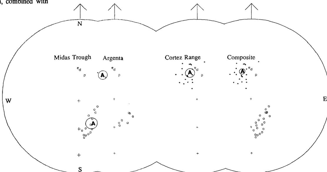
Figure 3. Equal-area projections of site mean directions from Midas trough, Argenta rim, and Cortez Range and composite data. Open symbols refer to site mean direction plotted on upper hemisphere; asterisk indicates direction on lower hemisphere. A is mean direction; d, p, and e are dipole field, present Earth field, and mid-Miocene expected (from North America craton) directions in sampling area.
