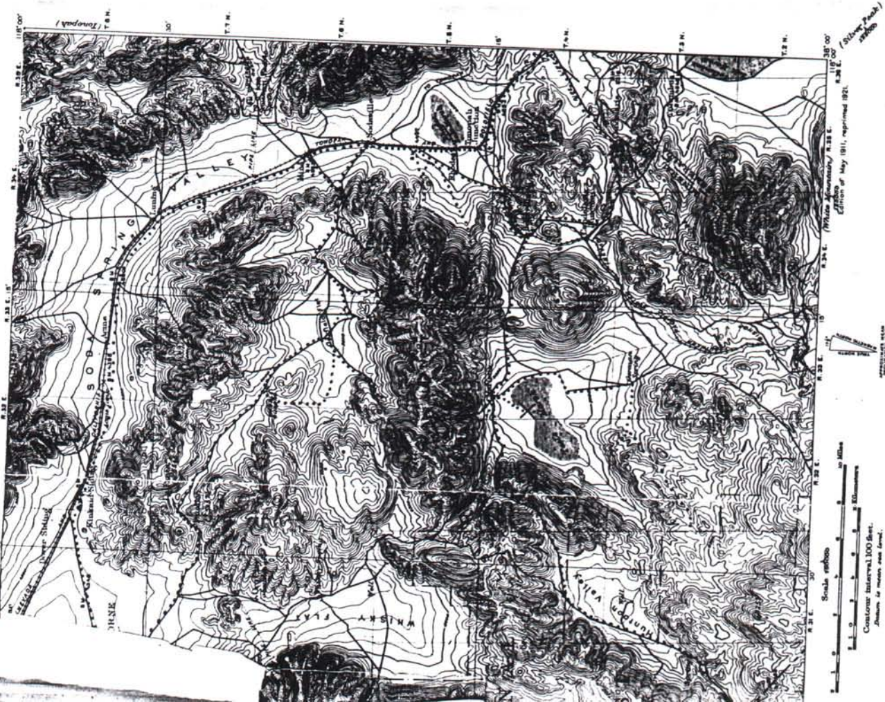
FIG. 1.—Topographic map showing the Excelsior Mountains and vicinity. The dotted lines indicate traverse and the crosses indicate the location of fissures. The earthquake fault occurs in the canyon north-north-west of Marietta. Taken from the Hawthorne quadrangle of the United States Geological Survey.
