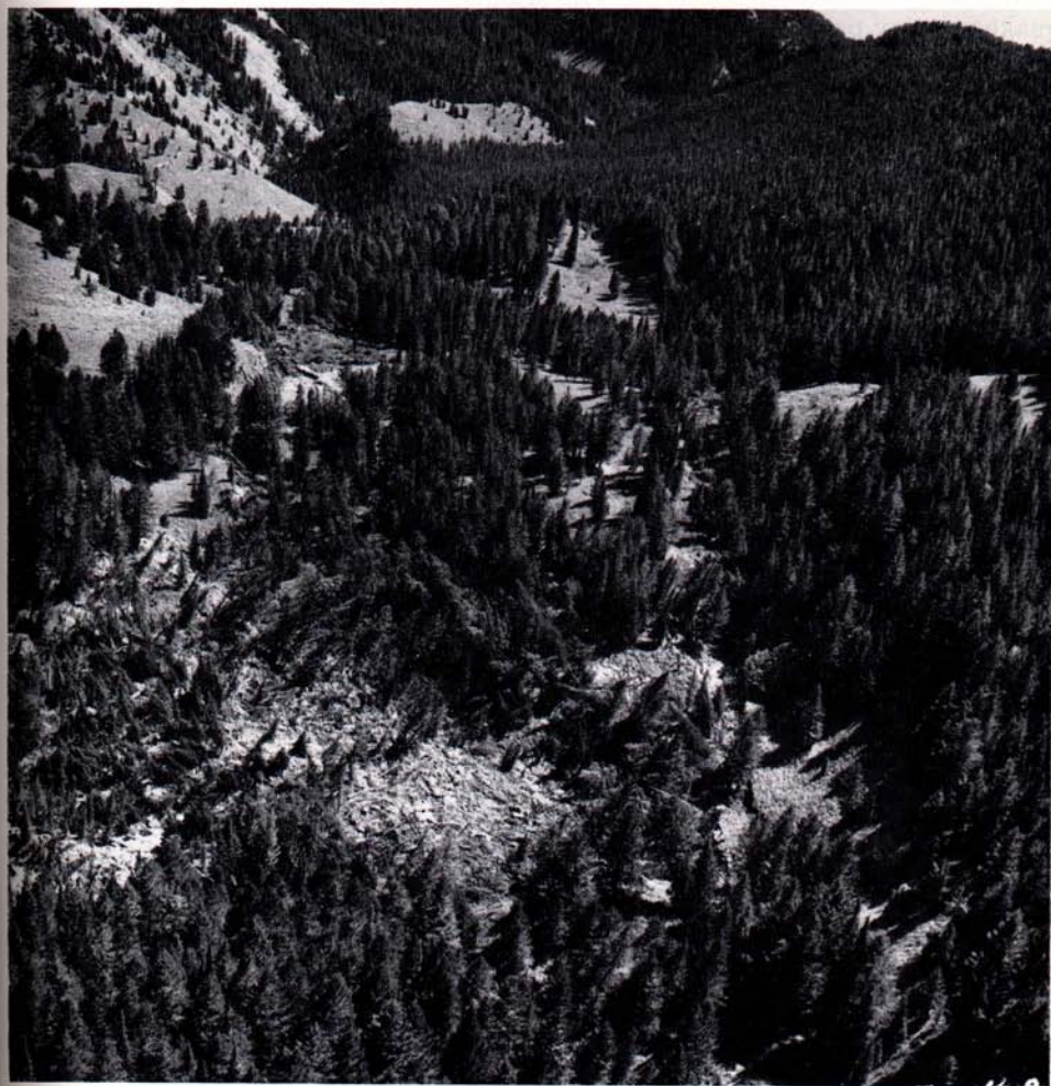
FIG. 9. Aerial view of the Kirkwood earthflow, Sept. 3, 1959, looking south in the direction of movement. The area of jumbled blocks and tilted trees in the foreground is near the head of the flow.
