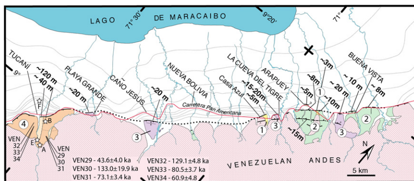
Fig. 10. Fault-truncated alluvial surfaces along northwestern flank of Andes are labeled 1, 2, 3, and 4 (values in circles) and, respectively, exhibit scarp heights of 3–5, \sim 10 , \sim 20 , and 120 m and record progressive late Quaternary uplift. Names, ages, and locations of boulders sampled for ^{10}\text{Be} TCN analysis near Tucaní are labeled. Scarp height measurements in meters. Photograph of 3-m-high scarp east of Arapuey is shown in Fig. 11A. Limits of profile measurements at Tucaní (stars) that are shown in Fig. 12 are labeled AB and EF, respectively. Lago de Maracaibo is at sea level and the contours outboard of the Andes are at 10-m intervals. Red line is Carretera Panamericana (highway). Bedrock in the Andes (stippled) and unfaulted alluvium outboard (northwest) of range front are undifferentiated.
