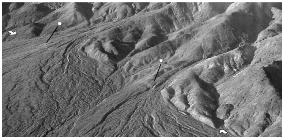
Figure 28. Oblique air photo of Indian Head fault trace (between arrows) along west flank of Indian Head Peak. Perspective of photo is annotated in Figure 24. Older elements of active fan preserve fault scarps (circle and star). Channel margin is dextrally offset \sim 6 m along fault trace (star).
