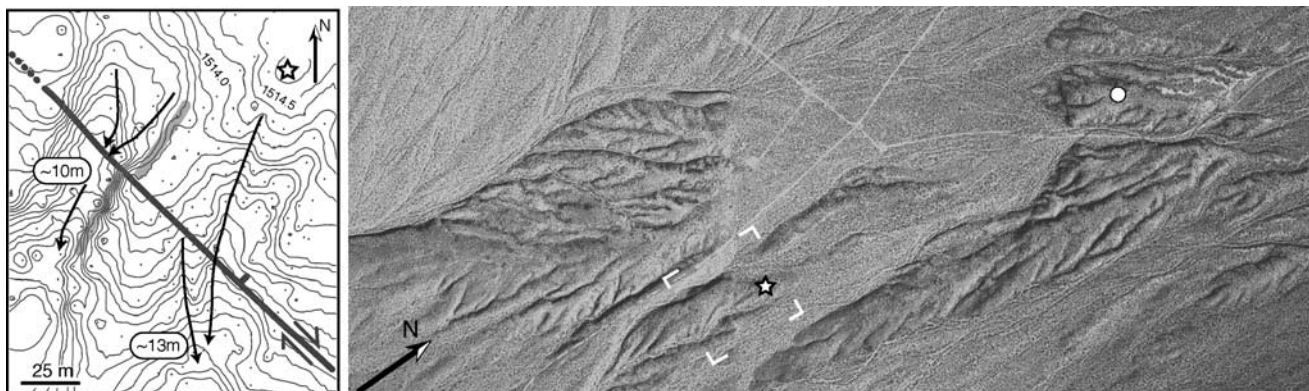
Figure 26. Aerial photo and 0.25 m contour map of dextral channel and channel margin offsets along subparallel strands of the Gumdrop fault in Soda Springs Valley. Brackets in air photo outline area of topographic map. Arrows delineate channels and flow directions. A channel margin (shaded) and beheaded channel are offset ~10 and ~13 m, respectively. Another dextral channel offset of about ~10 m is adjacent to white dot. UTM coordinate (UTM NAD 27 CONUS) of point marked by stars is N4270043 E394623. Location also noted on map in Figure 24.
